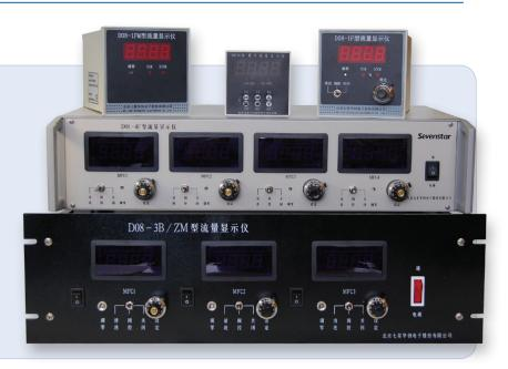
The D08 Flow Readout Box provides a power supply for one mass flow controller or mass flow meter. The D08 features a power supply, a flow setpoint and a flow display for mass flow controllers or mass flow meters and enables the user to set and display the flow for a single MFC or MFM. The D08 is offered in a compact digital- or analog-style readout box, desktop readout box, rack-type flow readout box or flow accumulator.
