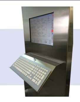
ESL has introduced a new touchscreen and keyboard modification for the Mattson RTP 2900 Front GUI panel. The original design has become obsolete and this new design allows the front panel at the side of the equipment to be used.
